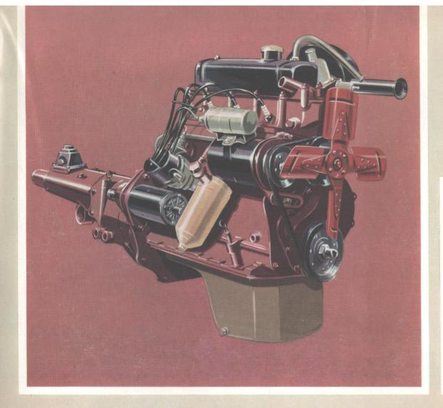
In standard form the 1622-c.c. o.h.v. engine transmits its power via a Borg & Beck clutch with hydraulic actuation and a four-speed gearbox with floor-mounted gear change lever. Now, for the first time, a Wolseley of medium size is offered with fully automatic transmission. The Borg-Warner Model 35 transmission brings exceptional
