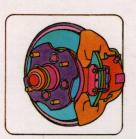
Front disc brakes—up where 80-85% of the braking action is. From freeway speeds these mighty binders stop the Sedan and Coupe
