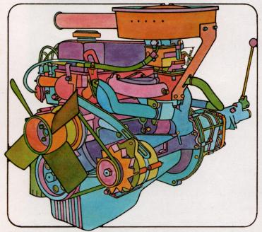
The 1200's hyper-efficient high-cam engine gets its 69 horses from just 71.5 cubic inches. It's internally modified for maximum emission control
