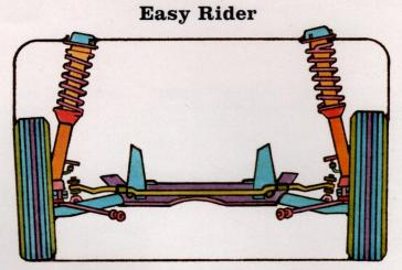
The 1200's suspension—independent strut type up front; semi-elliptic rear leaf springs. Ideal for multi-purpose machines this size and weight. Stable, sure-tracking for comfort and roadability.
