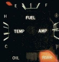
Low fuel indicator light. Handbrake warning light.
