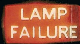
Stop and tail lamp failure warning light.
