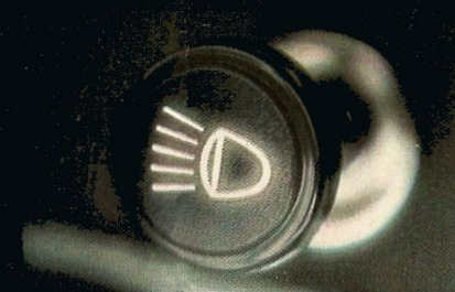
Light switch and rheostat panel light control.
