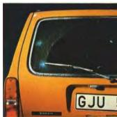
Volvo's estate car is better equipped to give the driver good rearward vision. The electrically heated rear window keeps frost and mist at bay and the wiper and washer make sure that road dirt or snow are swept away. These are both standard features on a Volvo 145.
