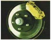
Volvo cars have power-assisted disc brakes all round. The 164 E has specially ventilated front discs to counteract fade. On all models, the handbrake operates on separate rear wheel drums.
