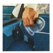
It's an easy matter to fold down the rear seat backrest and arrange a flat cargo area which is 74"/188 cm long. The backrest is dropped, from either side. The seat fixing mechanism has been improved for easier action and it now moves into place in one smooth movement.
