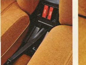
The handbrake is now located between the front seats in a housing which also incorporates the safety belt locks which are easier to use and easier to see, even at night, since they are illuminated. On the rear of the handbrake casing is an illuminated ashtray for the rear seat passengers.
