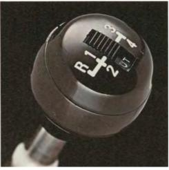
If you prefer a four-on-the-floor manual gearbox, your Volvo GL comes with a fully synchronized unit with electrically operated overdrive controlled by a switch built into the gear lever knob. A three-speed automatic with a six-position illuminated selector is optional.
