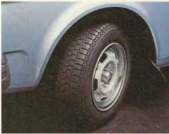
The chromium wheel studs of the Volvo GL hold new-design wheels and wide low profile steel-braced, radial ply tyres for better grip and less wear.
