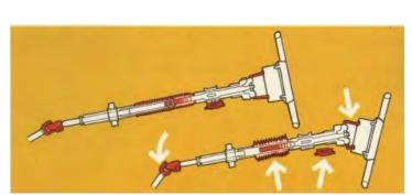
Volvo's steering wheel gives fivefold safety in the event of a headon collision: 1. The lower steering rod separates, 2. the steering column collapses, and 3, moves downwards away from the driver, 4, the wheel's anchorage to the column crumples, and 5. the wide bolstered hub spreads the impact.
