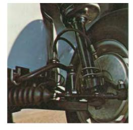
The new Volvos have rack and pinion steering which gives improved response and better stability and accuracy. With a turning circle diameter of only 32'2", the Volvo is a handy car in the city. In fact it can run circles round many smaller models.
