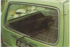
The new Volvo 245 tailgate window is electrically heated and has a wiper and washer as standard.
