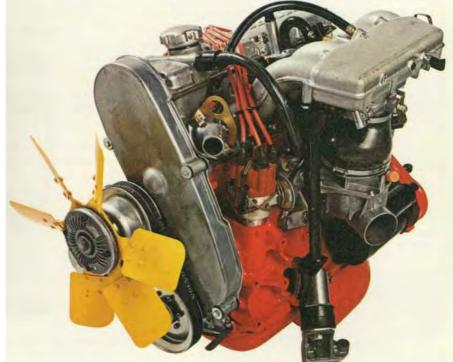
In its GL form, the new Volvo engine with overhead camshaft gives 123 hp DIN and thrives on 93 octane petrol. It's called the B 21 E; and features continuous fuel injection for smoother running and thriftier motoring. It has a solid-state ignition system which means there are no breaker points, meaning less maintenance, better performance and greater reliability.
