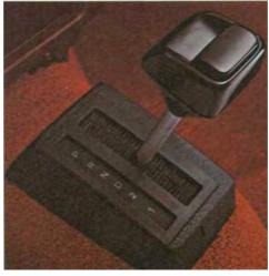
Researchers have shown that driving a car with an automatic transmission is often safer than driving one which has a manual gearbox. With an automatic, you simply have more time for the actual business of driving. Volvo's well-tested smooth changing automatic has a stubby gear lever and a sixposition selector with a quadrant which is illuminated at night.
