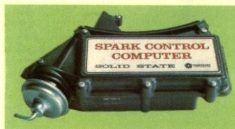
The brain of the Lean-Burn System is this electronic spark-control computer which responds to data from 8 sensors and instantly adjusts the timing of spark-plug firings to achieve the best combustion efficiency for all conditions. Since conditions are constantly changing, the computer is constantly making instantaneous adjustments in spark-plug firings. This results in good
