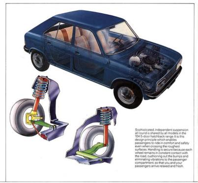
Mounted transversely, the engine is angled 72° to the rear. The space saved by adopting this engine layout can be utilised in the passenger compartment to offer more room for both passengers and their luggage, while keeping the overall length of the car to a minimum—just lift fullow [3,62m].
