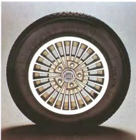
Alloy wheels reduce your car's unsprung weight and increase brake cooling. This 25 spoke 'sunburst' design polished aluminium alloy wheel is available with either a small (as illustrated) or large hub cap.
