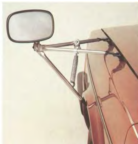
Quick and easy to fit to either wing without drilling the bodywork, the Volvo caravan mirror affords an excellent rear view.
