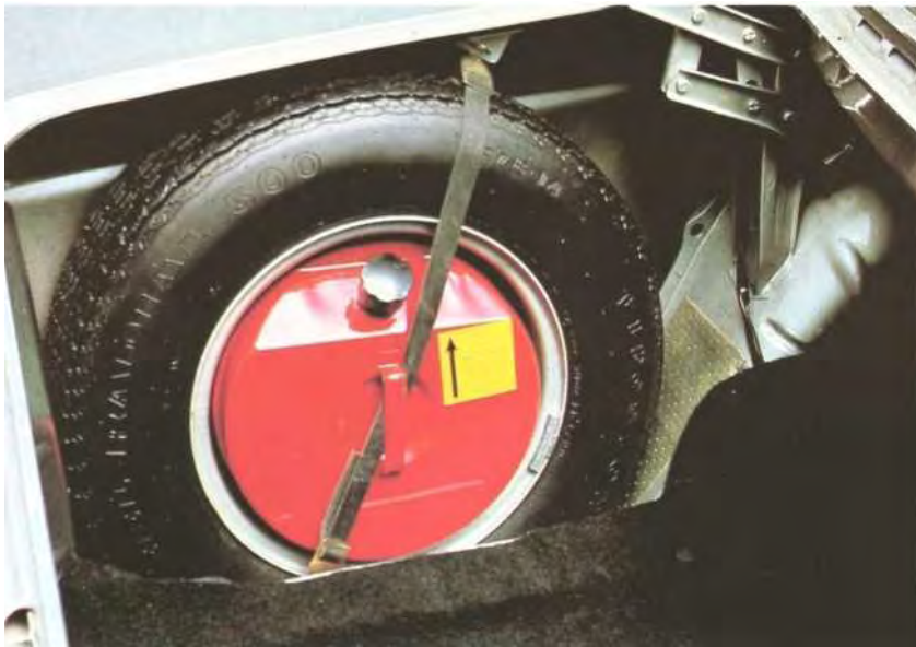
Volvo's space-saving fuel can fits snugly inside the spare wheel. Its capacity is 5 litres.
