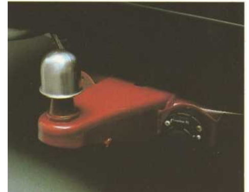
The sturdy, tubular steel tow bar is typical of the quality of all Volvo towing accessories. It will pull a load of 3,300 lbs (1500 kg) as will the alternative 'swing away' version.
