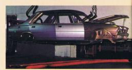
STEEL PANELS: All body parts are thoroughly degreased to remove oil deposited during the press operation and to ensure full adhesion of the protective finishes. Corrosion resistant zinc or galvanised plated panels are used in vulnerable areas or areas that would be difficult to protect after assembly.
