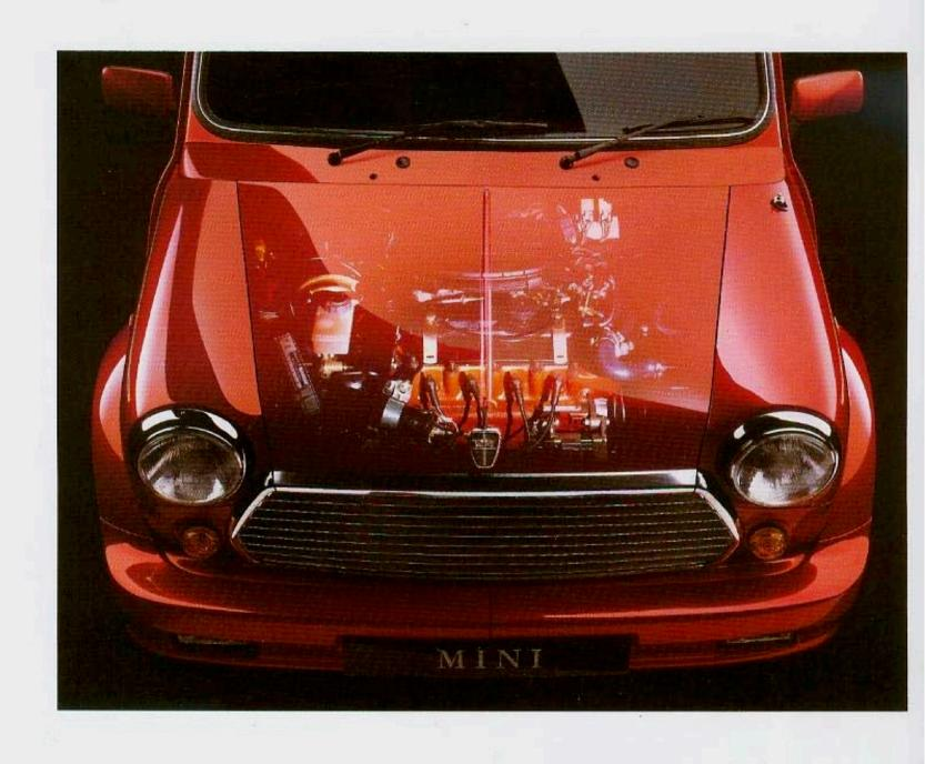
Punchy performance is combined with care for the environment; the Cabriolet's lively 63PS 1275cc fuel-injected engine is fitted with a three-way catalyst.
