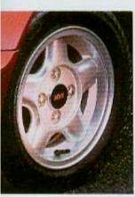
Giving an edge to that legendary bandling, the Cabriolet is fitted with 'Revolution' alloy wheels with 175/50 x 12 low profile tyres.
