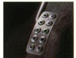
The drilled accelerator pedal is the classic racing design of the 1930's, and will be appreciated by drivers who like to heel and toe.
