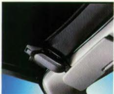
The two latches fastening the hood to the header rail are easily released.
