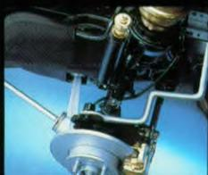
squarely on the tarmac. The MGF's trump card is its outstanding ride quality – with Hydragas® units interlinked front to rear soaking up the bumps and completely eliminating the 'fidgetiness' which often flaws compact sports cars.
