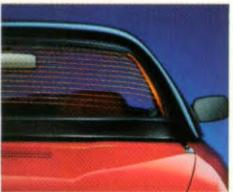
For all-weather visibility, the optional hard top is fitted with a heated rear screen.
