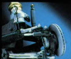
The MGF's mid-engine layout is exploited to the full with classic double wishbone suspension front and rear. Classic, because it's better than any other suspension at keeping the wheels at right angles to the road and the tyre tread
