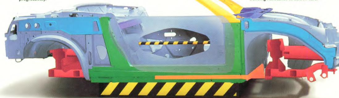
The strong sideframe (GREEN) and steel tubes inside the windscreen pillars (YELLOW) give equivalent bending resistance to saloon cars.
