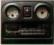
The 20 watts per channel electronic stereo radio/cassette player also has RDS.
