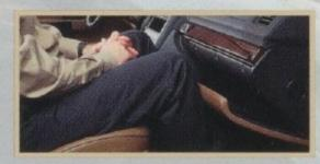
Range Rover's glove compartment can easily hit the front-seat passenger's knees when opening, restricting storage-area access.
