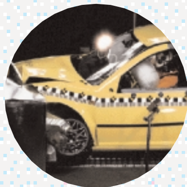
Rigorous crash testing simulates a front offset impact. Even at this speed, the survival zone remains largely intact.
