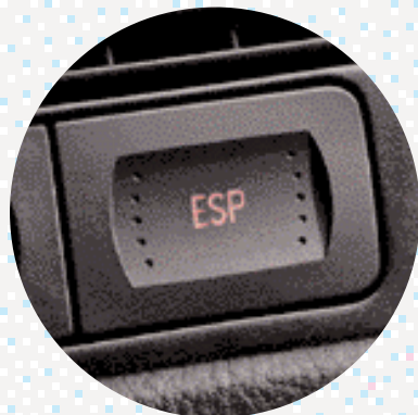
The Electronic Stabilisation Programme – ESP – helps to prevent losing control in unstable driving conditions.
