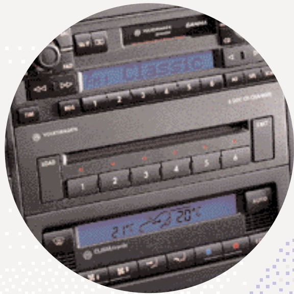
Standard on Sport and 'V' range, the dash-mounted 6 CD autochanger is available as a factory-fitted option on all other models.
