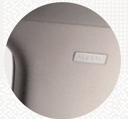
Roof-mounted airbags help protect the head from injury during a side impact.
