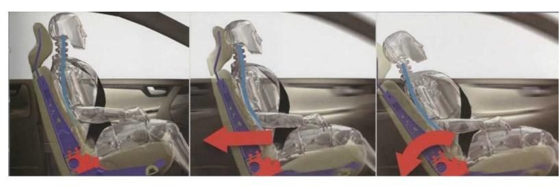
WHIPS (Whiplash Protection System) reduces the strain on the spine and neck in rear-end collisions. It is integrated in the front seats and is activated if a rear impact is sufficiently severe.
