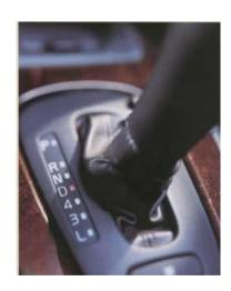
The five-speed adaptive automatic monitors your driving style and then automatically selects one of two gearshift modes: 'Sport' for faster shifts down and higher performance, or 'Economy' for lower fuel consumption and cleaner emissions.
