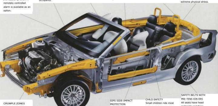
The front and rear crumple zones dissipate and distribute incoming collision forces so as to reduce the physical strain on the occupants.
