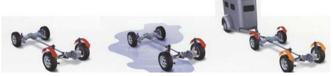
When braking, the car disengages drive to the rear wheels the moment you touch the brake pedal, preparing itself to maximise control and roadholding.
