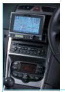
>> Satellite navigation unit A fully integrated navigation unit, built into a DIN size housing, it is ideally suited to the 307 with a double DIN aperture.
