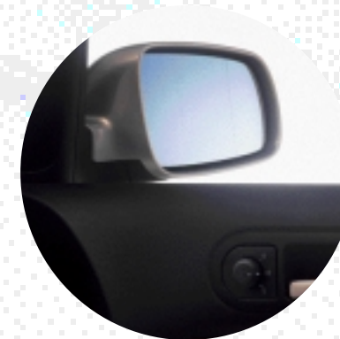
For greater all round vision, the electrically-adjustable door mirrors are also heated and fitted with blue tinted glass. Standard on Match models and above.
