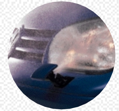
The retractable headlight washer system provides a highly effective method of removing dirt for improved night-time visibility.
