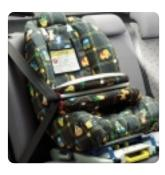
\*Please note that this seat should only be fitted in the front seat if the passenger airbag has been disabled.
