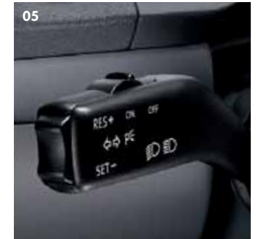
05 Cruise control can be set at speeds over 19 mph to maintain a constant speed. So even on long journeys you can have a high degree of relaxation. Optional on S, Sport, GT FSI/GT TDI and GTI models.
