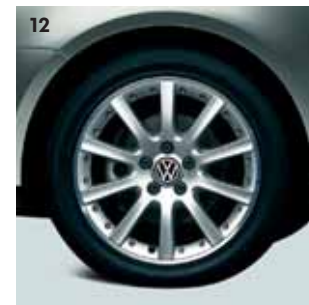
12 'Grand Prix' design 7J x 17 light alloy wheels with 225/45 R17 tyres. Optional on SE, Sport and GT FSI/GT TDI models.
