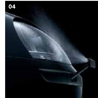
04 The Winter pack offers comfort and safety during the coldest months. The Winter pack includes electrically heated front seats, heated windscreen washer jets, headlight washers and a low washer fluid level warning light. Optional on all models.
