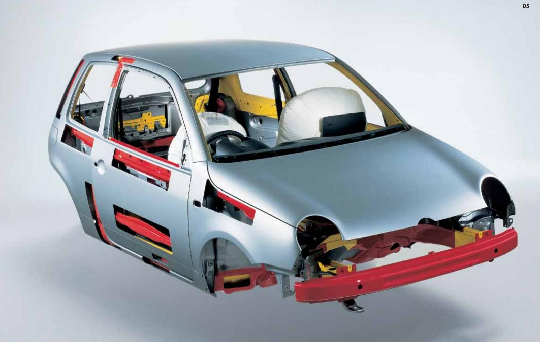
When designing a small car, safety is an important element. The chassis is extremely rigid and is equipped with crumple zones to absorb impact. The Lupo is a fine example of strength through design. This is evident when driving the Lupo, as its torsional rigidity improves handling and roadholding.
