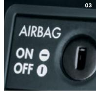
**03** The front passenger airbag can be deactivated, to allow the use of a rear facing child seat, by the simple turn of a key.
