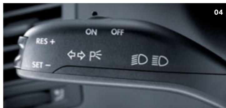
04 A simple push of a button will activate the cruise control and hold a desired speed whether you go uphill or downhill.
