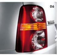
of Should you have to brake in an emergency situation, the hazard warning lights are activated automatically, helping to give advanced warning to other road users.
