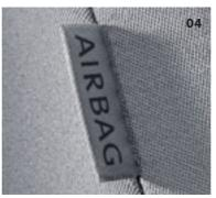
O4 Side airbags provide greater protection for the driver and front passenger, whilst the curtain airbag system protects the front and second row passengers.
