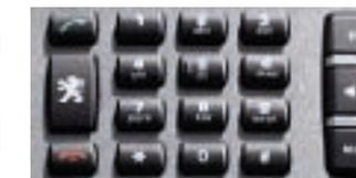
Make and answer your calls using the keypad on the central console, the control on the steering wheel or the voice-recognition function.
