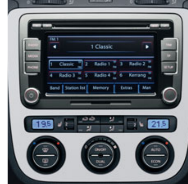
The optional RCD 510 touch-screen radio/dash-mounted MP3 compatible six CD autochanger with eight speakers and AUX-in socket for connection to external multimedia source e.g. iPod and MP3 player.
