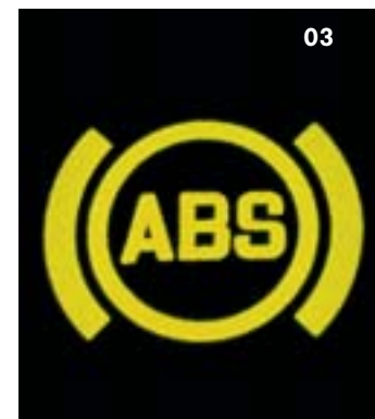
03 The Anti-lock Braking System (ABS) prevents the wheels from locking, even under severe braking.
