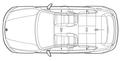
All dimensions in millimetres. Luggage compartment capacity (as per VDA standard): 330 to 1,150 litres. Model shown here is a BMW1 Series 5-door.
