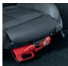
Powder-type fire extinguisher
