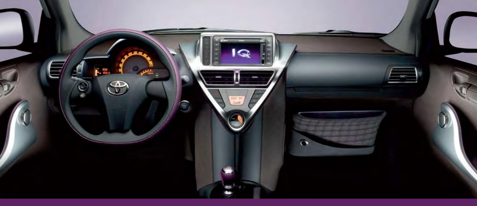
We haven't reinvented the wheel but challenged its traditional design. As a result, the steering wheel shaft is angled to give the driver more legroom. And to save space on the centre console, the steering wheel has been fitted with audio controls, so you can choose your favourite track without taking your eyes off the road.
