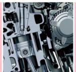
Clean power. Toyota's powerful yet environmentally friendly diesel engine technology. Common rail direct injection adjusts pressure, timing and volume as you drive, injecting finely atomised fuel at high pressure into the combustion chamber for the best performance.
