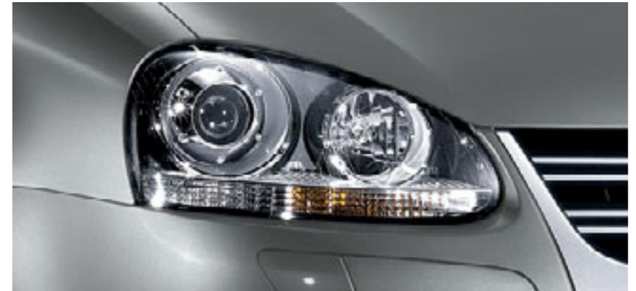
**Gas discharge (Xenon) dipped beam headlights** with automatic range adjustment improve visibility and the headlight washer system ensure they stay clean. Optional on all models.
