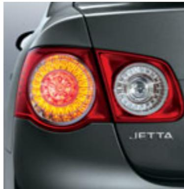
The **rear lights utilise LED technology** which react faster than conventional bulbs and provide clearer, brighter light.
