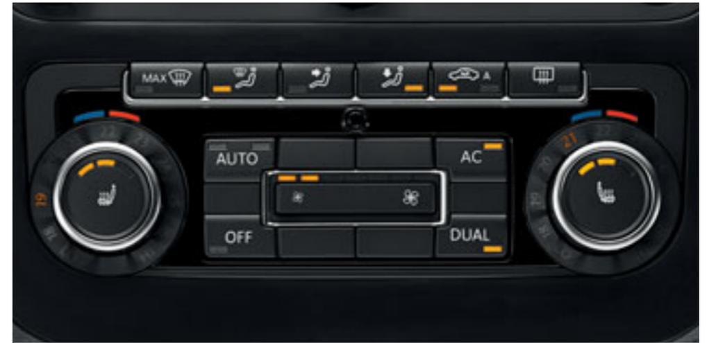
The **2Zone electronic climate control** with automatic air recirculation function is fully automatic to retain a precise internal temperature. It also benefits from a twin zone setting that allows the driver and front passenger up to 4°C difference in their chosen temperature settings. Optional on all models. Heated front seats form part of the Winter pack, optional on all models.
