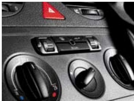
'Climatic' air conditioning.
