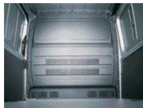
Full height steel bulkhead.
