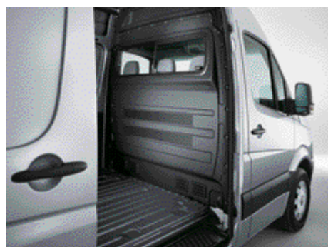
Bulkhead pack A. Shows optional second sliding door.
