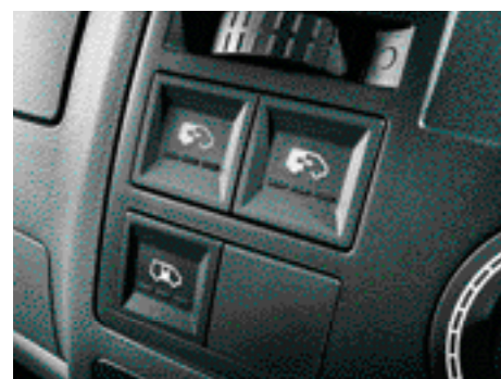
Electrically operated side sliding doors.
