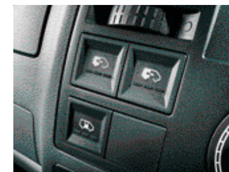
Electrically operated side sliding doors.
