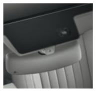
Safety when raining: the rain sensor adjusts the frequency of the windscreen wipers automatically to the intensity of rainfall.
