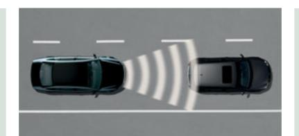
The side scan system helps you if you want to change lane safely at speeds over 37 mph. The system warns you of any road users in your blind spot via a warning light within the wing mirrors and an audible warning within the vehicle.
