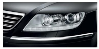
Bi-Xenon headlights: for dipped and main beam, with dynamic curve lighting, headlight washers and LED daytime running lights (standard on 6.0 W12 4MOTION). Built-in motors swivel the powerful headlights in the direction of travel, improving illumination ahead and to the edge of the road, helping you drive more safely, especially when cornering or turning. Separate LED daytime running lights switch on automatically with the ignition.
