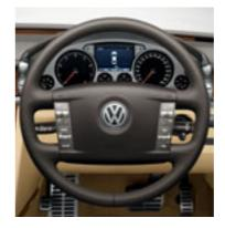
Multifunction heated leather trimmed steering wheel: offers excellent grip, looks extremely stylish and enables easy operation of the audio functions, cruise control, Multifunction computer, and optional telephone preparation.
