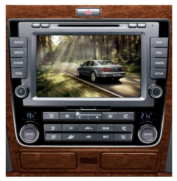
TV reception with teletext: enables you to watch both analogue and digital television transmissions in excellent picture and sound quality, when your Phaeton is stationary. A port enables you to use other external devices, for example an MP3 player.
