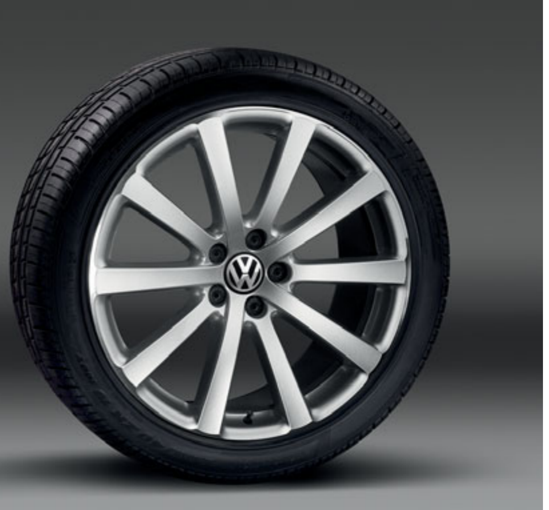
'Omanyt' design 9J x 19 alloy wheels with 255/40 R19 tyres including flat tyre indicator. Standard on R Line models.
