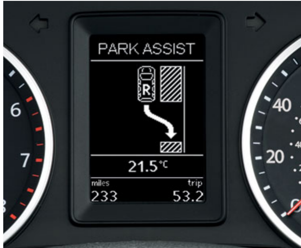
When driving past a parking space at up to 19 mph, the optional Park Assist with ultrasonic front and rear parking sensors, compares the space available, which can be as little as 1.1 m longer than the length of the Tiguan. If the space is suitable, the Park Assist parallel parking assistant automatically controls the steering as soon as you engage reverse gear. All you have to do is operate the accelerator, clutch and brake, while keeping a good lookout. Parking sensors also assist in less challenging parking manoeuvres by emitting both audible and visual signals, alerting the driver to any obstacles in the way: the closer you are to an obstacle the faster the sound frequency. The Optical Parking Display extends the functions of the parking sensors by indicating your position on the vehicle's audio display during parking (either in monochrome on RCD 310 or colour on RCD 510 and DVD navigation system). Optional on all models.
