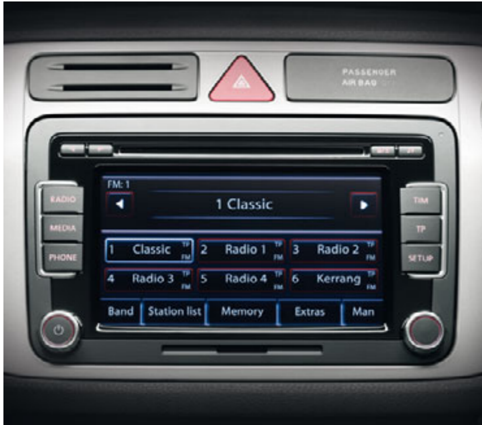
The RCD 510 touch-screen radio/dash-mounted MP3 compatible six CD autochanger with eight speakers and AUX-in socket for connection to an external multimedia source (e.g. iPod and MP3 player). Optional on S and standard on all other models.
