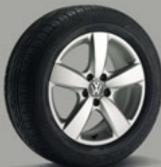
'Tunis' design 7J x 17 alloy wheels with 235/55 R17 tyres including flat tyre indicator. Standard on Escape and optional on S models.
