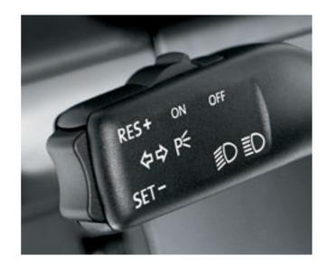
**Volkswagen Genuine Cruise control** Cruise control is an electronic aid for controlling your vehicle's speed. It helps you keep to speed limits, especially on long journeys. The reset function allows automatic acceleration after braking or changing gear.
