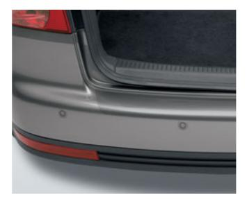
**Volkswagen Genuine Rear parking sensors** Make parking safer, easier and more convenient with these parking sensors. Automatically activated when reverse gear is engaged. Where applicable, the intelligent setup function recognises your towbar as not being an obstacle. Price excludes painting.
