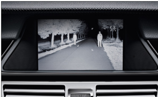
With Night View Assist Plus, an infrared image of the area normally illuminated on main beam can be seen on the central display
