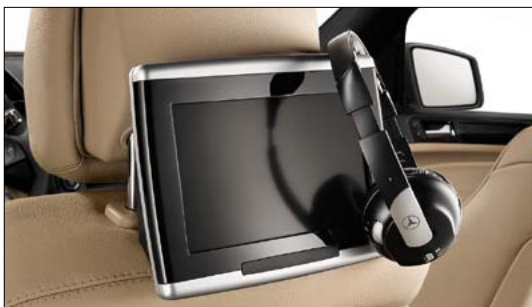
The rear seat entertainment system includes 8-inch colour screens for watching DVDs or playing games consoles
