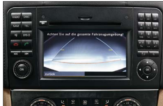
The reversing camera captures the area immediately behind the car
