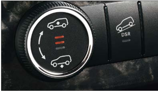
The GL's ride height can be raised or lowered via a dial in the centre console
