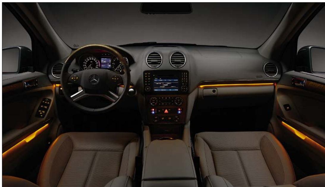
The ambient interior lighting comprises narrow strips of LEDs in the dashboard and doors and offers a choice of five brightness levels that can be selected via the menu in the instrument display
