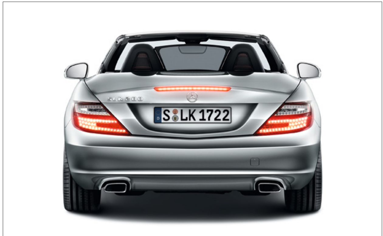
The adaptive brake lights increase safety by flashing during heavy braking, immediately alerting those behind
