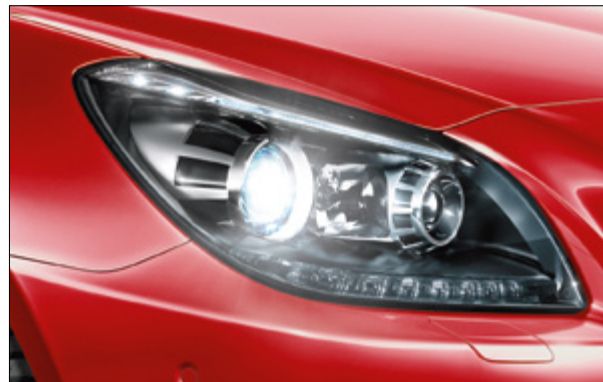
The Intelligent Light System adapts automatically to different roads and conditions
