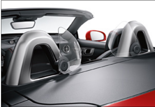
Airguide wind deflector, comprising twin Plexiglas® panels
