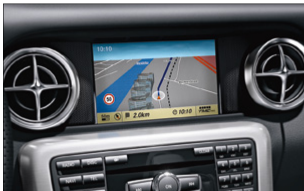
Speed Limit Assist shows the current speed limit in the instrument panel and in the central COMAND Online display
