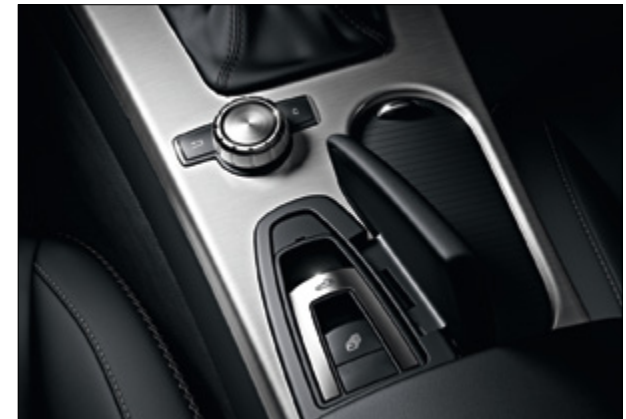
Roof controls and central controller
