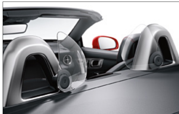
The innovative Airguide wind deflector significantly reduces draughts with the roof open
