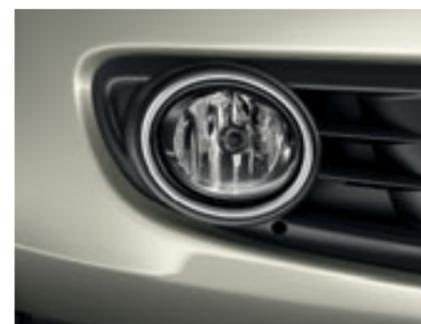
Chrome trimmed front fog lights add a striking look to the front of all Sportline models and include a static cornering function that illuminates the road when indicating or turning at low speed, as well as providing additional safety in bad weather or where there is poor visibility.
