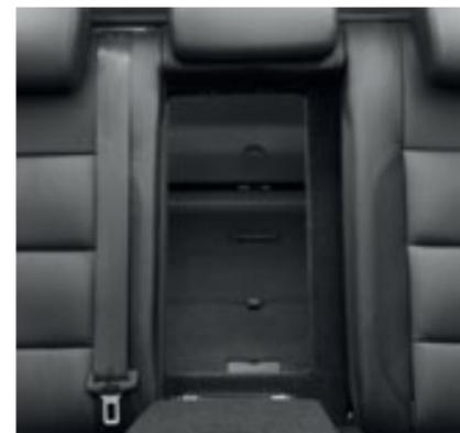
When the rear centre armrest is folded down, it provides a useful **load-through facility**, enabling you to transport skis, snowboards and other long objects easily and conveniently.
