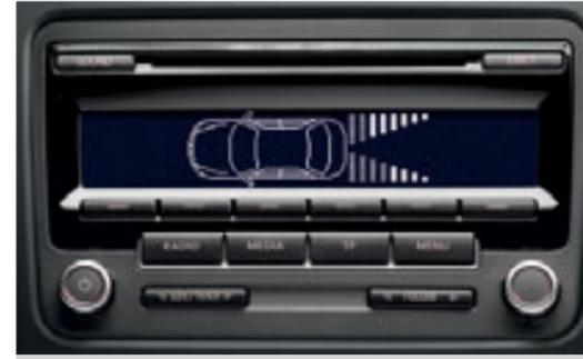
**Front and rear parking sensors** help with parking by emitting both audible and visual signals: the closer you are to an obstacle the faster the sound frequency. In addition, an **Optical Parking Display** shows your position on your audio system's display. Optional on all models.
