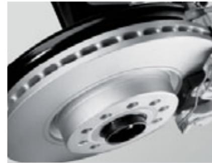
The front (ventilated) and rear discs brakes deliver excellent thermal performance, even if there is a sharp rise in temperature of the brakes.
