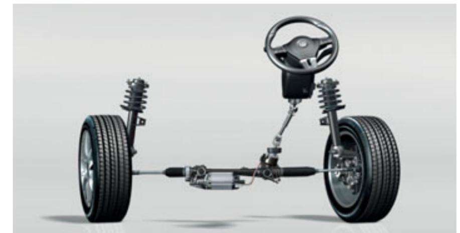
The electro-mechanical **power-assisted, speed-sensitive steering** adapts with the help of variable servo support to suit your driving speed. Power-assisted steering provides greater comfort and is more responsive.
