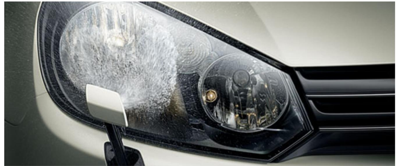
Headlight washers form part of the **Winter pack**, along with heated front seats, a low washer fluid warning light and automatically heated windscreen washer jets. Optional on all models.
