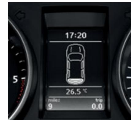
The **multifunction computer (Highline)** shows such information as average speed, fuel consumption and driving time. BlueMotion Technology manual models also feature a visual gear change recommendation which helps in achieving optimum fuel consumption.
