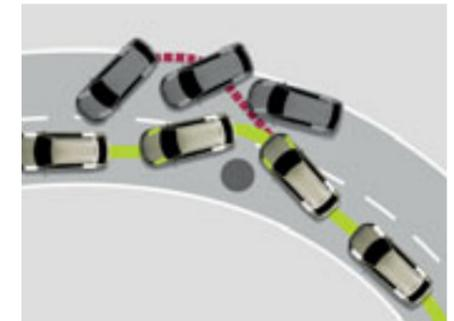
The **Electronic Stabilisation Programme (ESP)** recognises critical driving situations and reacts in milliseconds by targeting brake and management systems, controlling the speed of individual wheels and helping to bring the vehicle under control.
