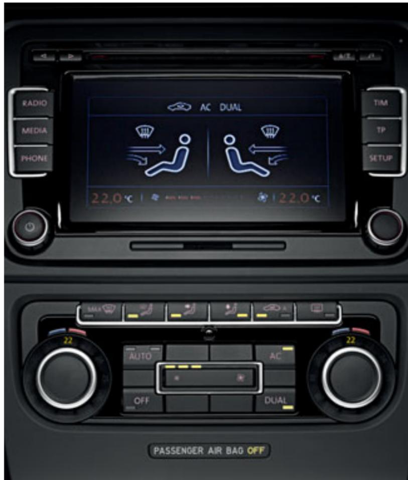
**2Zone electronic climate control air conditioning** features dual zone control for the driver and front passenger, allowing each to select their individually preferred temperature. A sensor monitors the exterior air quality and, if necessary, automatically activates the air recirculation function. Optional on all SE and Sportline models.
