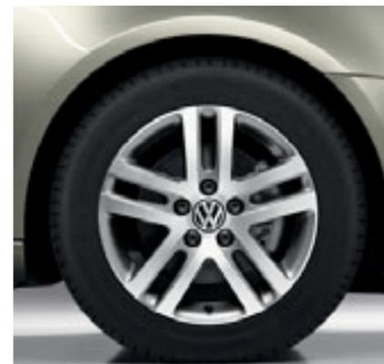
Stylish 16 inch 'Atlanta' alloy wheels with 205/55 R16 tyres and anti-theft wheel bolts provide a distinctive look to the exterior. Standard on all SE models. SE BlueMotion Technology and Sportline BlueMotion Technology models are fitted with 205/55 R16 low rolling resistance tyres as standard.
