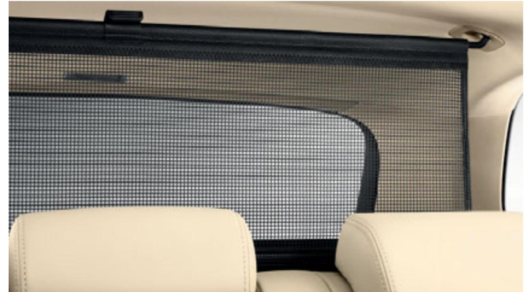
Keep your luggage safely in place with the **retractable net partition**. This option has a two position usage and can be used with the seats upright or when folded flat. Optional on all models.
