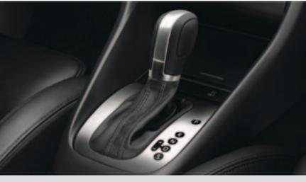
The **DSG dual-clutch gearbox** shifts smoothly and imperceptibly into the pre-selected next gear, within a split second, without disrupting the power. Such extremely short reaction times and direct response behaviour make sporty acceleration even more fun. The DSG gearbox is not only highly dynamic, but also extremely fuel-efficient.
