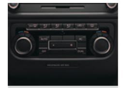
The 2Zone electronic climate control with automatic air recirculation system features dual zone temperature control for the driver and front passenger, enabling each to select their individually preferred temperature.
