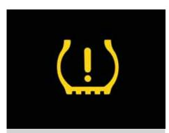
In the event of a change in air pressure, the **flat tyre indicator** symbol appears in the multifunction display, advising the driver to rectify the situation.
