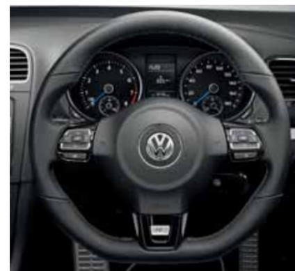
The **leather trimmed three-spoke multifunction steering wheel** with 'R' logo, 'Gloss Black' inserts and contrast stitching enables you to control the multifunction computer and radio without taking your hands off the wheel. It is also equipped with paddle shift when the DSG direct shift gearbox is specified. Contrast stitching also adorns the gear knob and leather handbrake to complete the sporty look.
