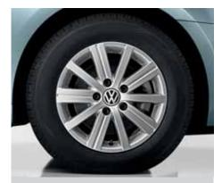
15 inch 'Wellington' alloy wheels with low rolling resistance tyres help to reduce the BlueMotion's fuel consumption.
