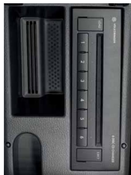
In addition to your RNS 510 touch-screen navigation/DVD radio system you can also specify an armrest-mounted six CD autochanger, in lieu of MDI (Multi Device Interface), allowing you hours of uninterrupted listening pleasure. Optional on all models except S and BlueMotion.
