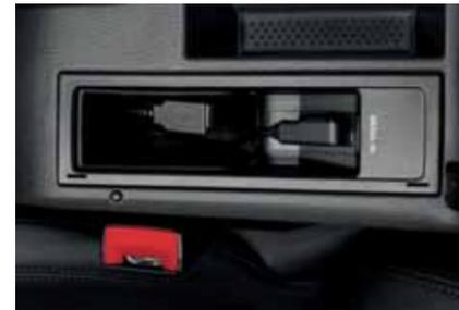
The front centre armrest features both a Multi Device Interface (MDI) and an AUX-in socket with the facility to connect, charge and store a compatible iPod or USB device. The rear passengers also benefit from two rear air vents and two cup holders.
