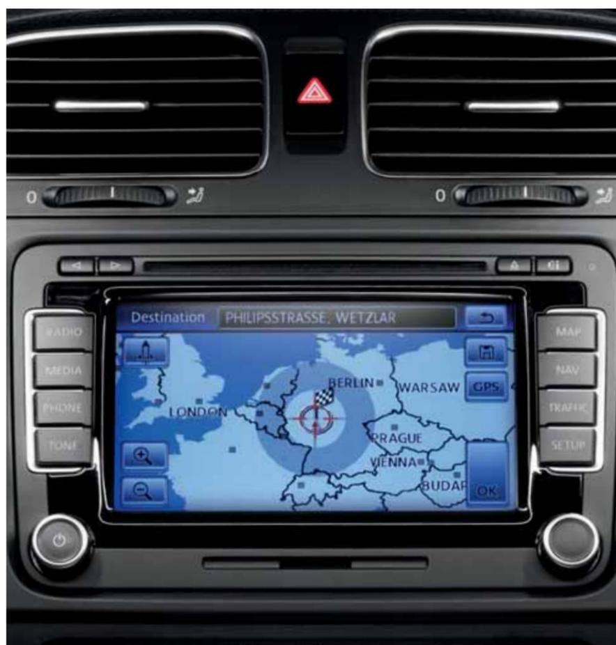
The RNS 510 touch-screen navigation/DVD radio system with integrated voice control will guide you to your destination using preloaded navigation data and includes a 6½ inch colour display. This state-of-the-art system responds to spoken voice commands for navigation, CD and radio functions. It also plays DVDs (when the vehicle is stationary) and music from the DVD drive, 30 GB hard drive or via an SD card. Optional on all models except S and BlueMotion.
