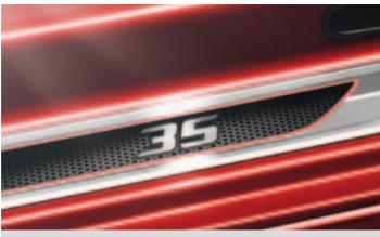
The **door sill strips** with a honeycomb pattern identifies your GTI as an anniversary model and protects the door sill area from scratches.
