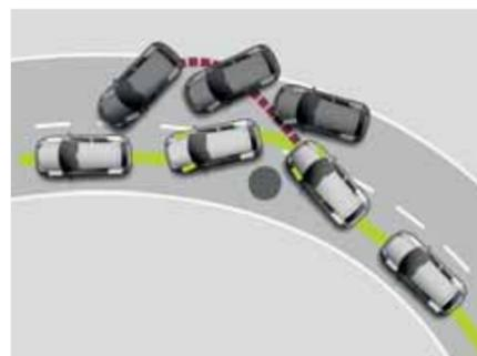
The **Electronic Stabilisation Programme (ESP)** recognises critical driving situations and reacts in milliseconds by targeting brake and management systems, controlling the speed of individual wheels and helping to bring the vehicle under control. As a result the vehicle achieves maximum directional stability.
