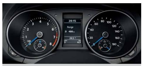
White instrument lighting and blue needles, enhance the sporty appearance, while the multifunction computer (Highline) provides important information as you travel, such as average speed and fuel consumption, exterior temperature, range of the fuel tank, and oil temperature. It also lets you know if the doors or boot are open.
