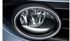
Front fog lights including static cornering function which illuminates when indicating or turning at low speed. Not only do they improve safety in the event of poor visibility, but with a chrome trimmed surround, they also provide a sporty finish.
