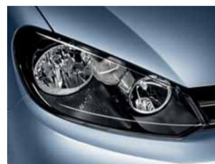
Range adjustable Halogen headlights with daytime running lights and integrated indicators flow seamlessly into the radiator grille, giving the Golf its distinctive appearance.
