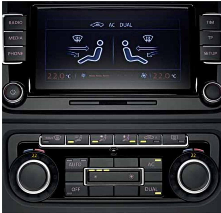
The **2Zone electronic climate control with automatic air recirculation system** features dual zone temperature control for the driver and front passenger, allowing each to select their individual preferred temperature. Standard on GTD, GTI, GTI Edition 35 and R models and optional on Match, Match BlueMotion Technology, GT and GT BlueMotion Technology models.
