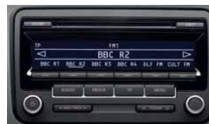
The RCD 310 radio/MP3 compatible CD player features eight speakers with an output of 4 x 20 watts. It also features an AUX-in socket for connection to an external multimedia source (e.g. iPod or MP3 player). Optional on S and BlueMotion and standard on all other models except Match and Match BlueMotion Technology.
