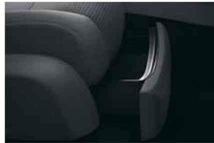
The **Storage pack** extends the Golf's numerous storage facilities even further to include drawers beneath the front seats, a net beneath the rear parcel shelf and a net on the boot floor. Optional on all models except S and BlueMotion.
