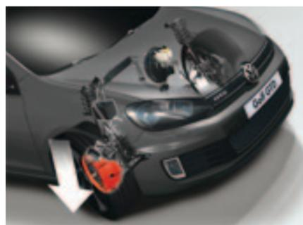
For the first time in the GTD, **Volkswagen's XDS system** which in conjunction with ESP, is designed to provide maximum grip and driving stability by helping to prevent loss of traction while cornering.
