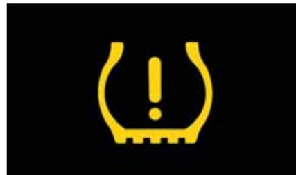
In the event of a change in air pressure, the **flat tyre indicator** symbol appears in the multifunction display, advising the driver to rectify the situation. Standard on GT, GT BlueMotion Technology and R, and optional on all other models.
