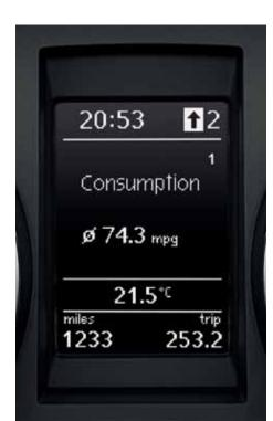
The multifunction computer (Highline) provides useful statistics about your journey, such as exterior temperature, average and current fuel consumption, average speed and estimated distance to refuelling. It also includes a visual gear change recommendation for optimum fuel consumption.
