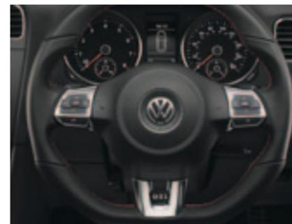
The **multifunction leather steering wheel** enables you to operate the radio system and multifunction computer without taking your hands off the wheel. When used in conjunction with the Direct Shift Gearbox (DSG), the gears can be changed easily from the steering wheel, using easy-grip paddles.
