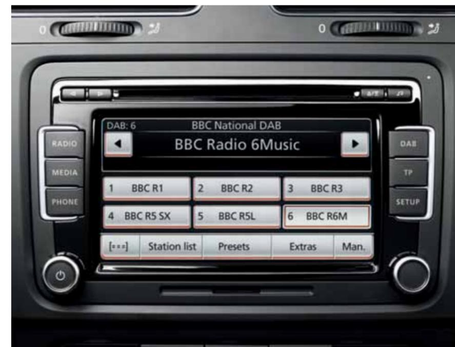
The RCD 510 touch-screen radio/dash-mounted MP3 compatible six CD autochanger features a large 6½ inch colour display, with intuitive menu navigation and touch-screen operation. It also features an AUX-in socket for connection to an external multimedia source (e.g. iPod or MP3 player) and an SD memory card slot. Standard on Match and Match BlueMotion Technology and optional on all other models.
