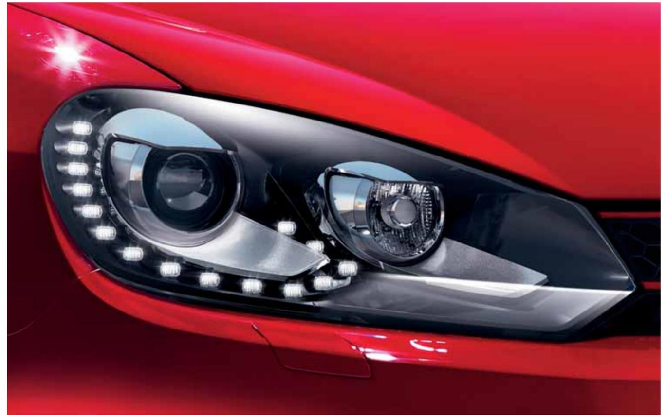
**Bi-Xenon headlights** feature dynamic curve lighting and automatic range adjustment providing better illumination of the road ahead, on bends and when turning off. LED daytime running lights ensure your vehicle is more visible to other road users. Standard on GTI Edition 35 and R and optional on GTD and GTI models.
