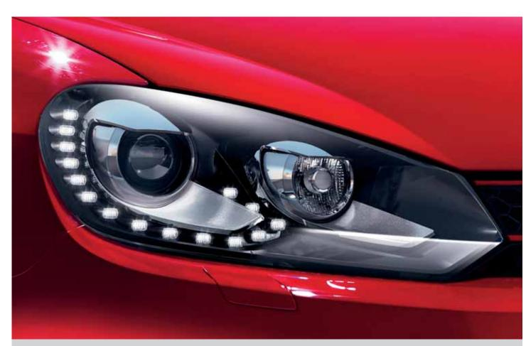
**Bi-Xenon headlights** feature dynamic curve lighting and automatic range adjustment providing better illumination of the road ahead, on bends and when turning off. LED daytime running lights ensure your vehicle is more visible to other road users. Standard on GTI Edition 35 and R and optional on GTD and GTI models.
