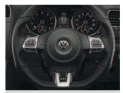
The multifunction leather steering wheel enables you to operate the radio system and multifunction computer without taking your hands off the wheel. When used in conjunction with the Direct Shift Gearbox (DSG), the gears can be changed easily from the steering wheel, using easy-grip paddles.
