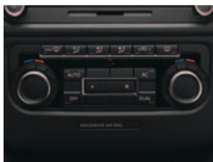
The **2Zone electronic climate control with automatic air recirculation system** features dual zone temperature control for the driver and front passenger, enabling each to select their individually preferred temperature.
