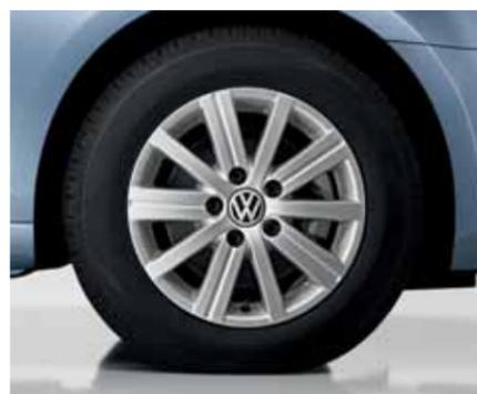
'Wellington' 6½J x 15 light alloy wheels with 195/65 R15 low rolling resistance tyres. Standard on BlueMotion models.
