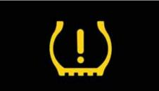
In the event of a change in air pressure, the **flat tyre indicator** symbol appears in the multifunction display, advising the driver to rectify the situation.
