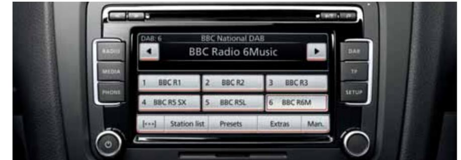
The RCD 510 DAB digital radio/dash-mounted MP3 compatible six CD autochanger features a large 6½ inch touch-screen colour display with intuitive menu navigation. Additional features include an AUX-in socket for connection to an external multimedia source, SD memory card slot and **Bluetooth telephone preparation** for HFP (Hands Free Profile) enabled telephones, allowing calls to be rerouted to your car's audio system.
