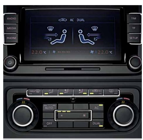
The **2Zone electronic climate control with automatic air recirculation system** features dual zone temperature control for the driver and front passenger, allowing each to select their individual preferred temperature. Standard on GTD, GTI, GTI Edition 35 and R models and optional on Match, Match BlueMotion Technology, GT and GT BlueMotion Technology models.
