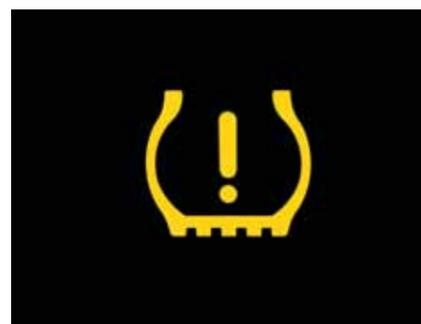
In the event of a change in air pressure, the **flat tyre indicator** symbol appears in the multifunction display, advising the driver to rectify the situation. Standard on GT, GT BlueMotion Technology and R, and optional on all other models.
