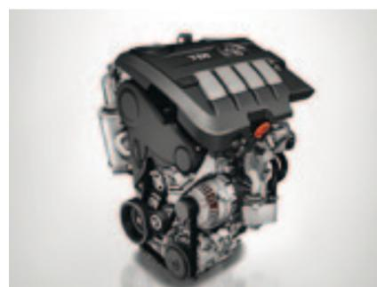
The GTD's **2.0 litre TDI 170 PS diesel engine** with common rail technology provides incredible torque and power, whilst still returning highly efficient fuel economy.
