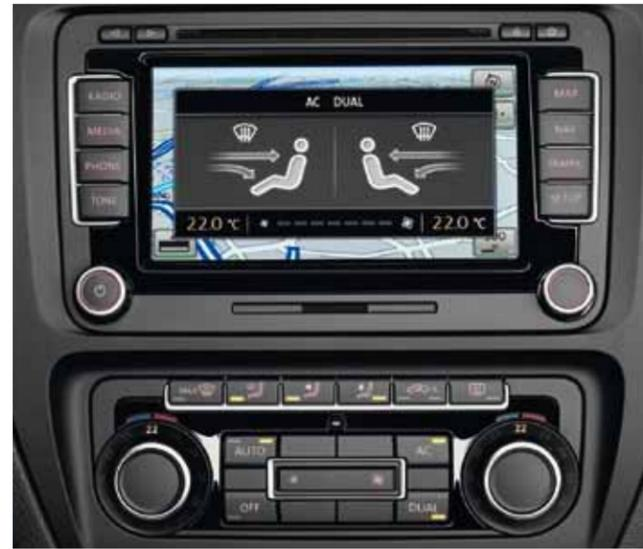
**2Zone electronic climate control with automatic air recirculation**, controls the temperature electronically and divides the interior into two different climate zones, enabling the driver and front passenger to adjust the temperature, air supply and distribution to suit their individual preference.
