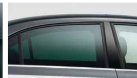
**Heat insulating tinted glass** from the B pillar backwards reduces sunlight by up to 65%, helping to ensure a pleasant temperature in the passenger compartment and also providing additional privacy.
