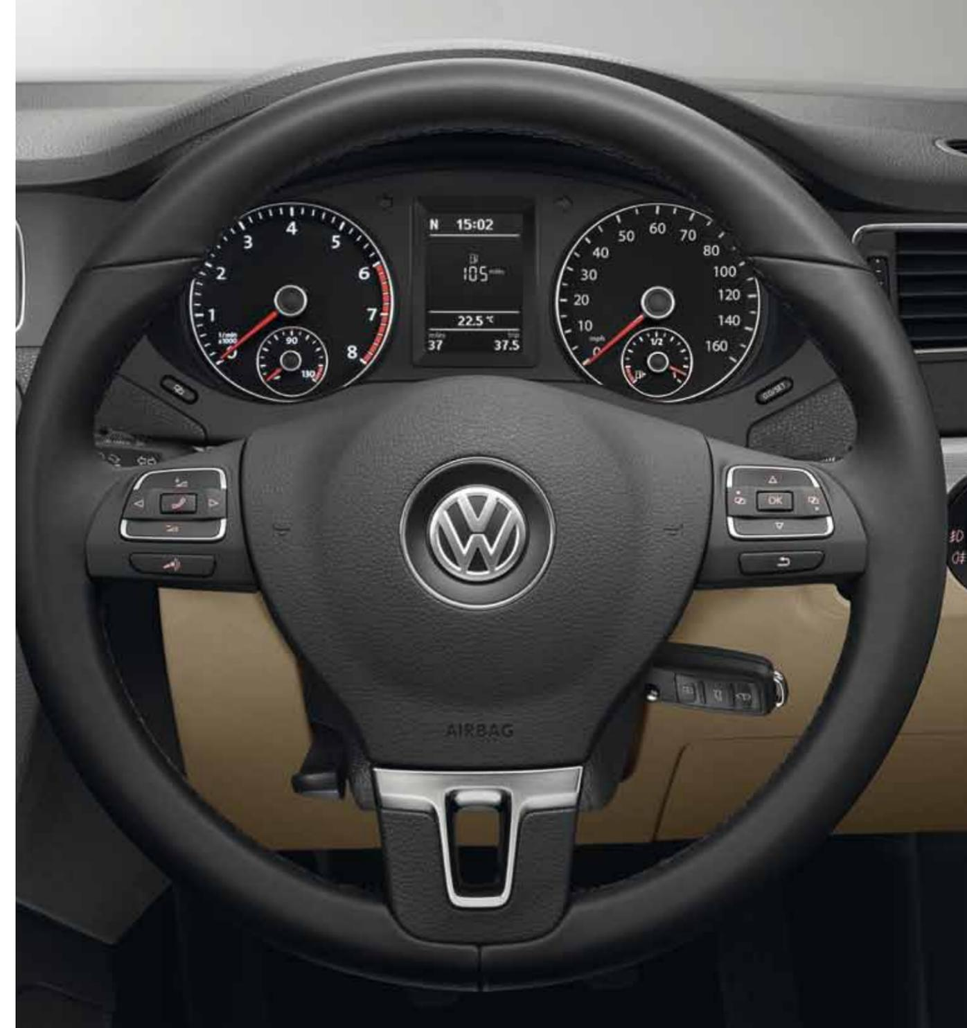
The **leather trimmed multifunction steering wheel** is fitted with ergonomically designed switches, making it easy to use the radio, in-car entertainment system and multifunction computer. Thanks to the height and reach adjustment of the steering column, the position of the steering wheel can also be set to your exact preferred driving position.
