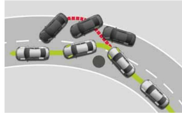
The **ESP (Electronic Stabilisation Programme)** recognises critical driving situations and reacts in milliseconds by targeting brake and management systems, controlling the speed of individual wheels and helping to bring the vehicle under control. As a result, the vehicle achieves maximum directional stability. A careful driving style is still essential, however, as even the Electronic Stabilisation Programme cannot defy the law of physics.
