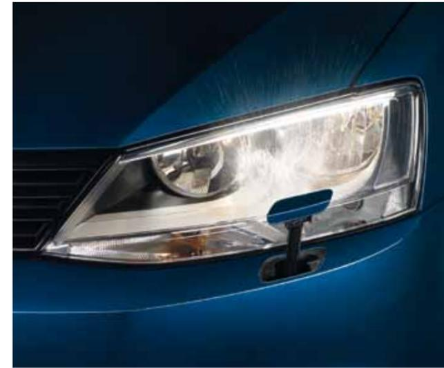
The **headlight washer system** forms part of the **Winter pack**, along with heated front seats, heated windscreen washer jets and low washer fluid warning light. This clever system will ensure that your headlights are kept clean of dirt and grime.
