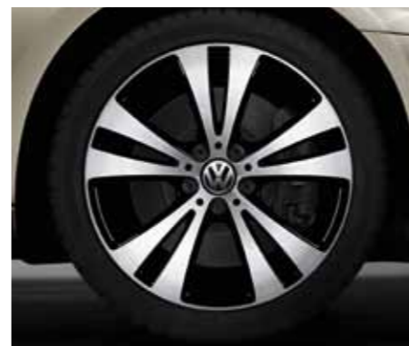
'Chicago' 8J x 18 with 235/40 R18 ContiSeal (self-sealing) tyres and anti-theft wheel bolts. Optional on all models.
