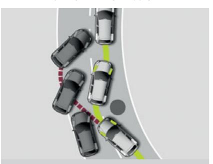
The ESP (Electronic Stabilisation Programme) recognises critical driving situations and reacts in milliseconds by targeting brake and engine management systems, controlling the speed of individual wheels and helping to bring the vehicle under control. As a result the vehicle achieves maximum directional stability.
