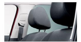
The two whiplash-optimised front head restraints not only ensure additional comfort, but also provide particularly effective support for the head and spine in the event of a collision.
