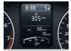
The multifunction computer (Midline) displays current fuel consumption figures on the display screen, and also makes recommendations for optimal gear changes on the 1.4 litre 85 PS and diesel models.
