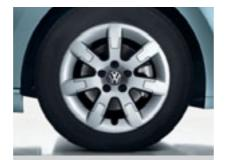
'Greenland' 51/2 J x 15 light alloy wheels with 185/60 R15 low rolling resistance tyres help to reduce the BlueMotion's fuel consumption. Standard on BlueMotion models.
