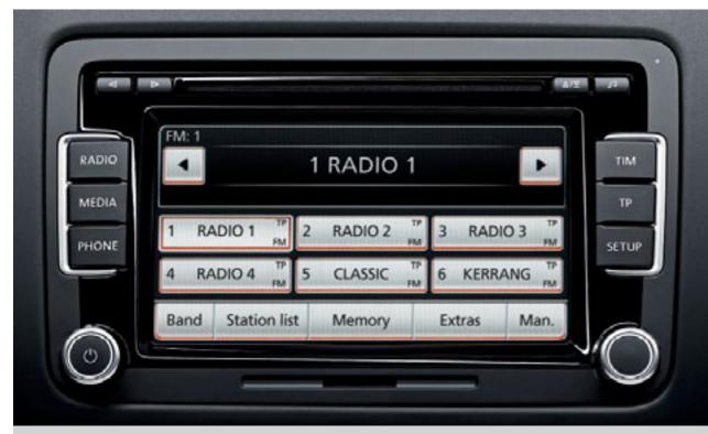
The RCD 510 touch-screen radio/dash-mounted MP3 compatible six CD autochanger features a large 6½ inch colour display, with intuitive menu navigation and touch-screen operation. It also features an AUX-in socket for connection to an external multimedia source (e.g. iPod or MP3 player) and an SD memory card slot. Optional on all models except S.
