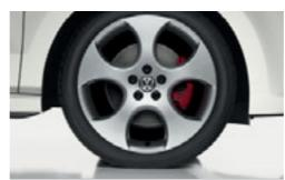
Standard 7½ J x 17 'Monza' alloy wheels with 215/40 R17 low profile tyres give the Polo GTI its purposeful image, the distinctive five spoke design revealing the red brake calipers behind.
