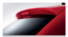
A high level third brake light integrated into the rear spoiler enhances aesthetics and improves vehicle safety.
