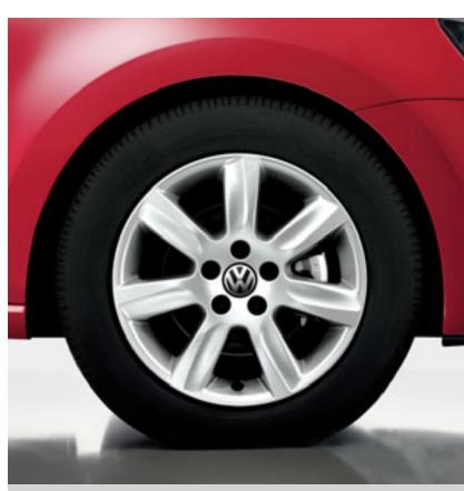
'Castille' 6J x 15 alloy wheels with 185/60 R15 tyres and anti-theft wheel bolts add a contemporary finishing touch to the exterior. Standard on Match models.
