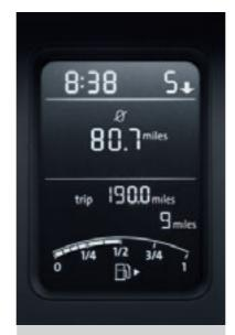
The multifunction computer (Midline) provides useful statistics about your journey, such as exterior temperature, average and current fuel consumption, average speed and estimated distance to refuelling. It also includes a visual gear change recommendation for optimum fuel consumption.
