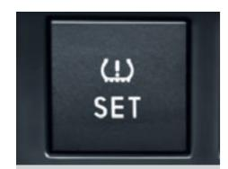
In the event of a change in air pressure, the tyre pressure indicator alerts the driver via a warning in the multifunction display. Not only does correct tyre pressure ensure a high degree of safety, but it also helps extend the life of the tyres and reduces fuel consumption.
