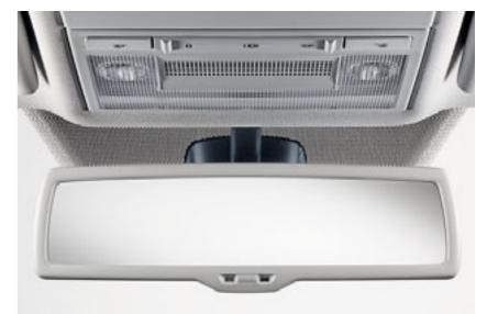
The **convenience pack** comprises an automatically dimming interior rear-view mirror which darkens when a following car's headlights are too bright, and rain sensor, which automatically activates and controls the windscreen wipers when it detects moisture on the windscreen. Optional on all models except S.
