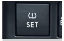
As part of the Sensor pack, the tyre pressure indicator will alert you to any change in tyre pressure via a warning in the multifunction display, advising you to rectify the situation.
