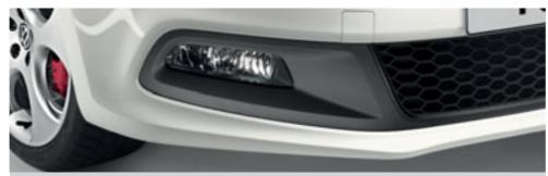
The **front fog lights** of the Polo GTI are neatly integrated into the lower front bumper. Not only do they improve safety in the event of poor visibility, but they also provide a sporty finish.
