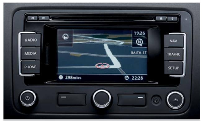
The RNS 310 touch-screen navigation/radio system features a 5 inch colour display for clear map navigation, guiding you to your destination using preloaded navigational data. The MP3 compatible single CD player will play music CDs even when the navigation system is being used, while music can also be played via the SD card slot. Optional on all models except S.
