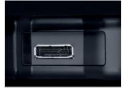
The MDI (Multi Device Interface) connects you to external audio sources, such as USB or iPod, which you can operate via the radio or optional navigation/radio system.
