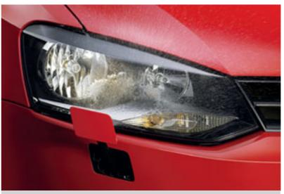
Headlight washers form part of the Winter pack, helping to improve safety in rain, snow and poor road conditions. Heated front seats provide comfort during cold weather, while heated windscreen washer jets help ensure visibility is maintained in the winter months. A low washer fluid warning light is also included. Optional on all models.
