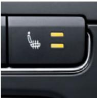
Heated front seats, which form part of the Winter pack, greatly increase comfort levels, especially in winter, providing heat faster than the car's heating system. Optional on all models.
