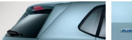
The rear spoiler not only enhances the BlueMotion's dynamic lines but also helps to reduce the vehicle's air resistance, and in turn reduces fuel consumption.
