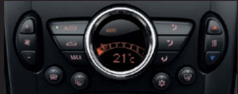
7. Automatic air conditioning
