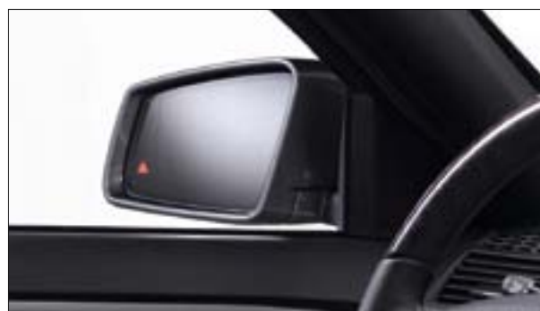
Active Blind Spot Assist warns the driver of potentially dangerous lane changes
