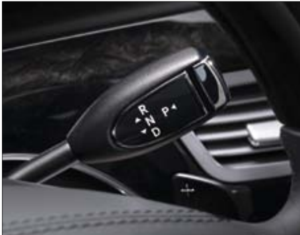
The Direct Select gear shift lever on the steering column
