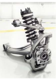
AMG Ride Control sports suspension with Adaptive Damping System and three suspension modes
