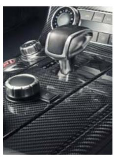
AMG carbon-fibre interior trim with genuine carbon fibre for the centre console
