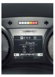
AMG instrument cluster with seven-LED upshift indicator for manual mode
