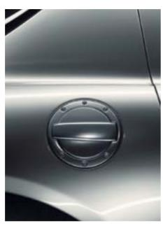
Screw-type solid metal fuel filler cap
