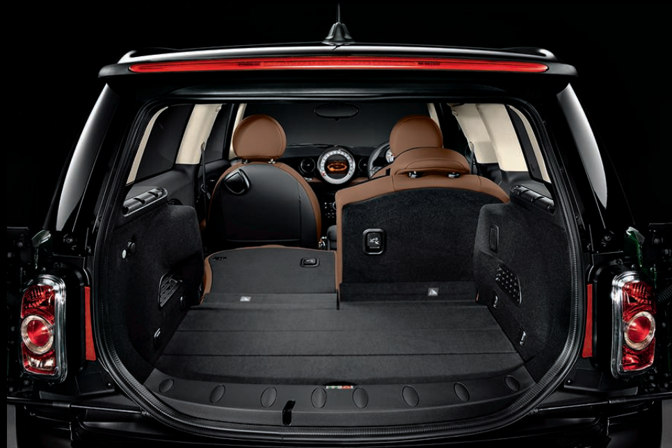
The rear seat backrests in MINI Clubman models fold down separately. The flat load floor makes for easier loading and unloading. Items can be secured to the four lashing eyelets.
