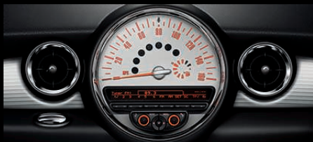
The large speedo is positioned in the middle of the instrument panel, and incorporates various warning lights and the fuel gauge.
