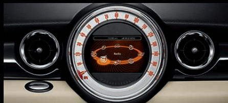
If the MINI Navigation system or MINI Radio Visual BOOST is fitted, then the speedo runs round the outside of the central round instrument.
