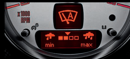
3. Rain sensor and automatic lights-on
