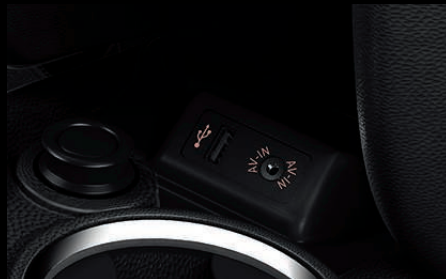
3. Basic Bluetooth telephone preparation with USB audio interface
